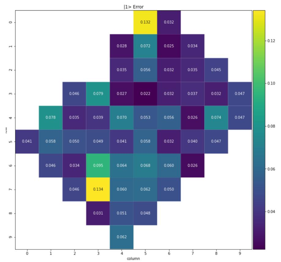
Simultaneous All Qubits  $|0\rangle$  Readout Error
